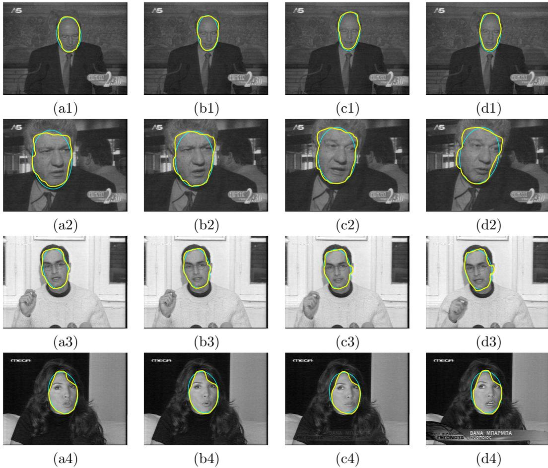
Fig. 16. Face tracking results of the proposed rule-based method, without applying the model-based term: the final results (contours) are illustrated in bold, whereas the shape prior (ellipse), to be further applied (16), is shown in soft lines.
