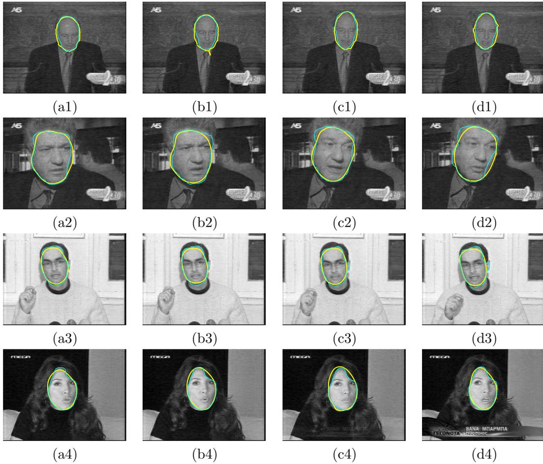
Fig. 17. Face tracking results of the proposed method, after applying the model-based (shape prior) term: the final contours are illustrated in bold, whereas the results obtained without the shape prior (15), are shown in soft lines.
